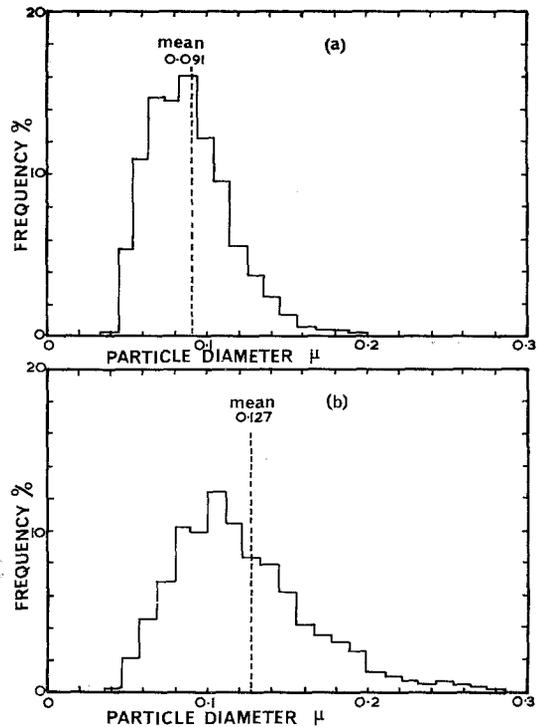
Figure 6 Planar size distribution curves for carbides in 1.2% chromium 0.2% carbon steel tempered for 10 h at 700° C. Etched for 8 sec (a), and 60 sec (b).
