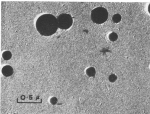
Figure 2 Copper/2 vol % SiO<sub>2</sub> electropolished and shadowed at 50°.
