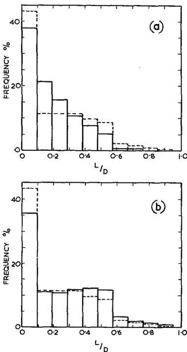
Figure 5 Histograms of shadow lengths on replicas of 1.2% chromium 0.2% carbon steel tempered for 10 h at 700° C. Etched for 8 sec (a), and 60 sec (b).
