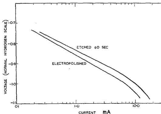
Figure 10 Cathodic polarisation curves in 3%  $\text{NaHCO}_3$ , 0.1%  $\text{H}_2\text{SO}_4$  solution of 1.2% chromium 0.2% carbon steel tempered for 10 h at 700° C.
