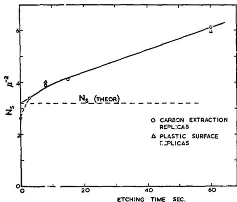
Figure 9 Dependence of number of particles per unit projected area ( $N_s$ ) on time of etching for 1.2% chromium 0.2% carbon steel tempered for 10 h at 700° C.
