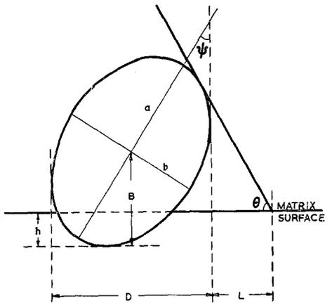
Figure 12 Geometry of shadowing an ellipsoidal particle. Section normal to the matrix surface containing the direction of shadowing.
