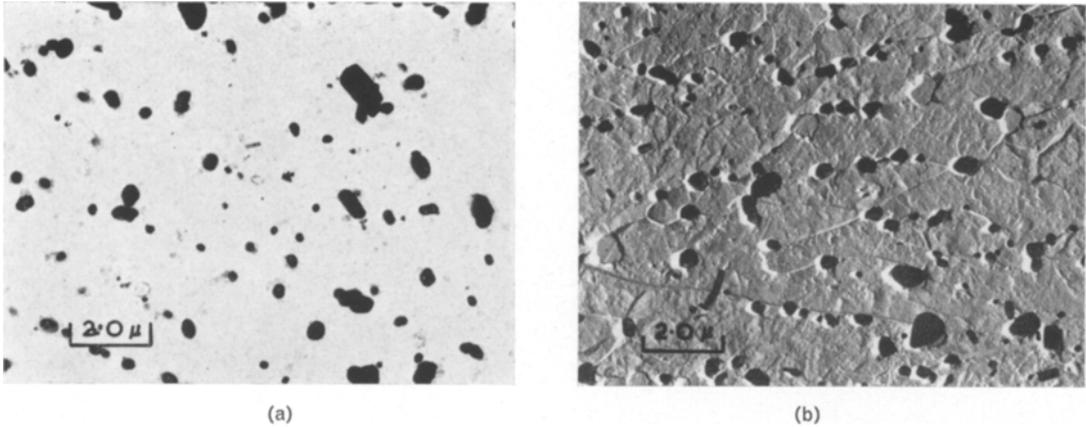
Figure 1 2.4% chromium 0.2% carbon steel tempered for 384 h at 700° C; (a) plain extraction replica, (b) shadowed extraction replica.
