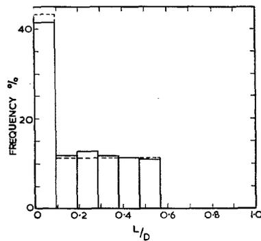
Figure 3 Histogram of shadow lengths on replicas of copper/2 vol % SiO<sub>2</sub>. Dashed curve predicted for randomly distributed spheres.
