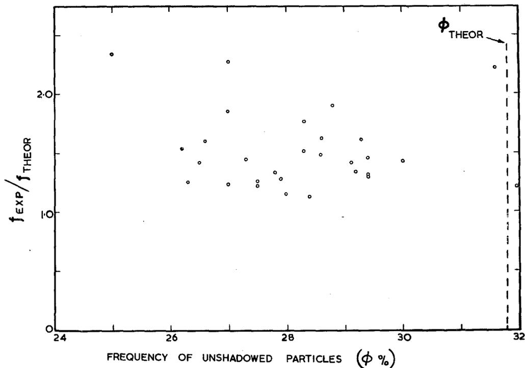
Figure 11 Relationship between ratio of experimental to theoretical volume fraction and frequency of unshadowed particles. Angle of shadowing  $50^\circ$ .
