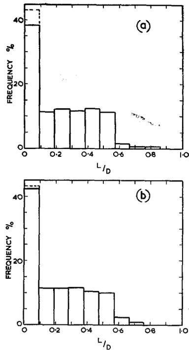
Figure 8 Histograms of shadow lengths on replicas of (a) 6.10% chromium 0.2% carbon and (b) 0.87% chromium 0.2% carbon steels tempered at 700°C.
